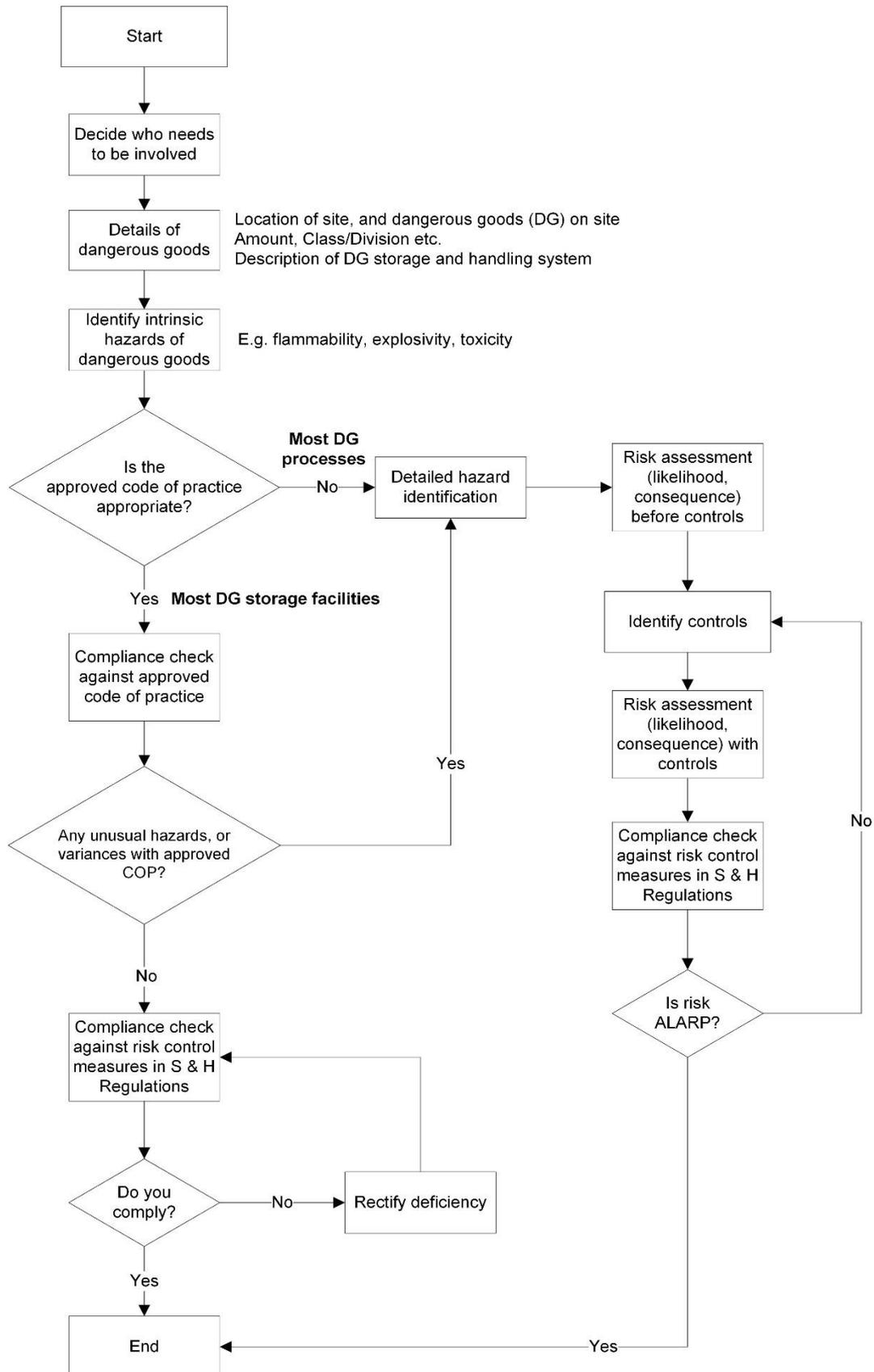
Figure 1 Flow diagram showing steps in hazard identification and risk assessment for dangerous goods storage and handling. Aligns with relevant sections of the dangerous goods risk assessment template
