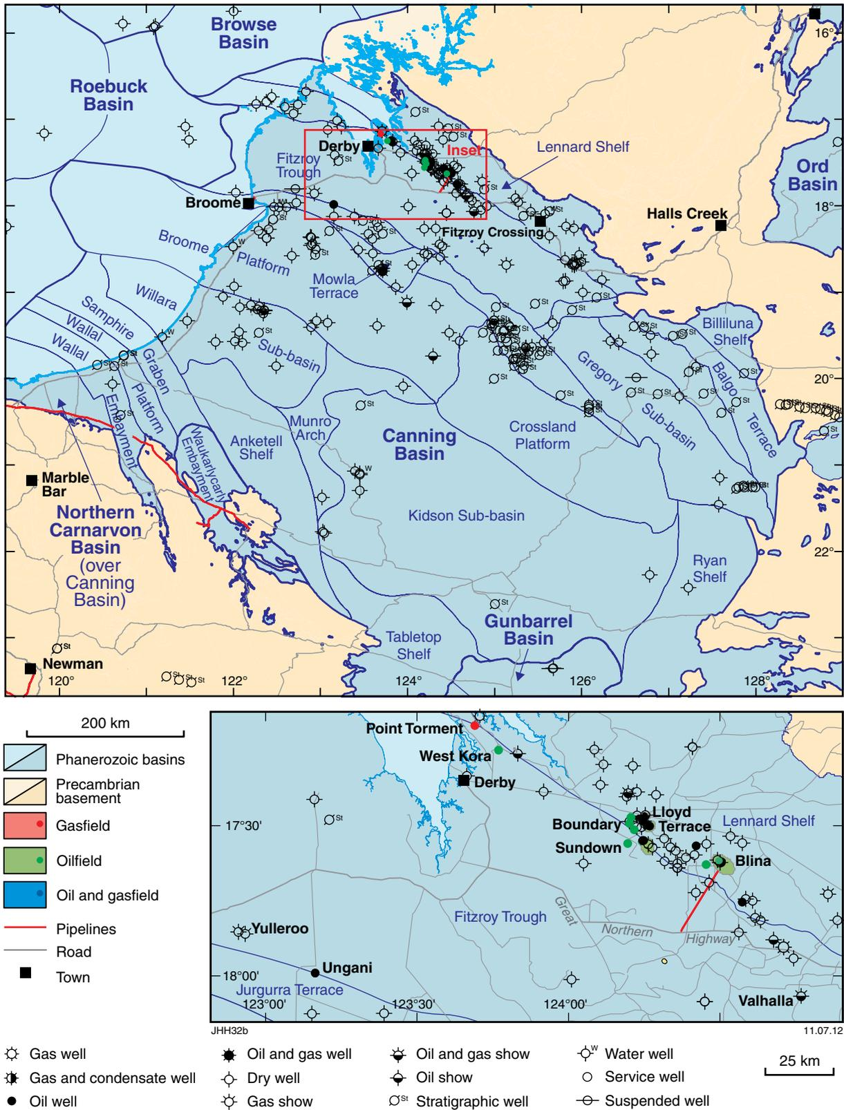
Figure 15. The Canning Basin, showing tectonic units, pipelines, fields and petroleum wells
