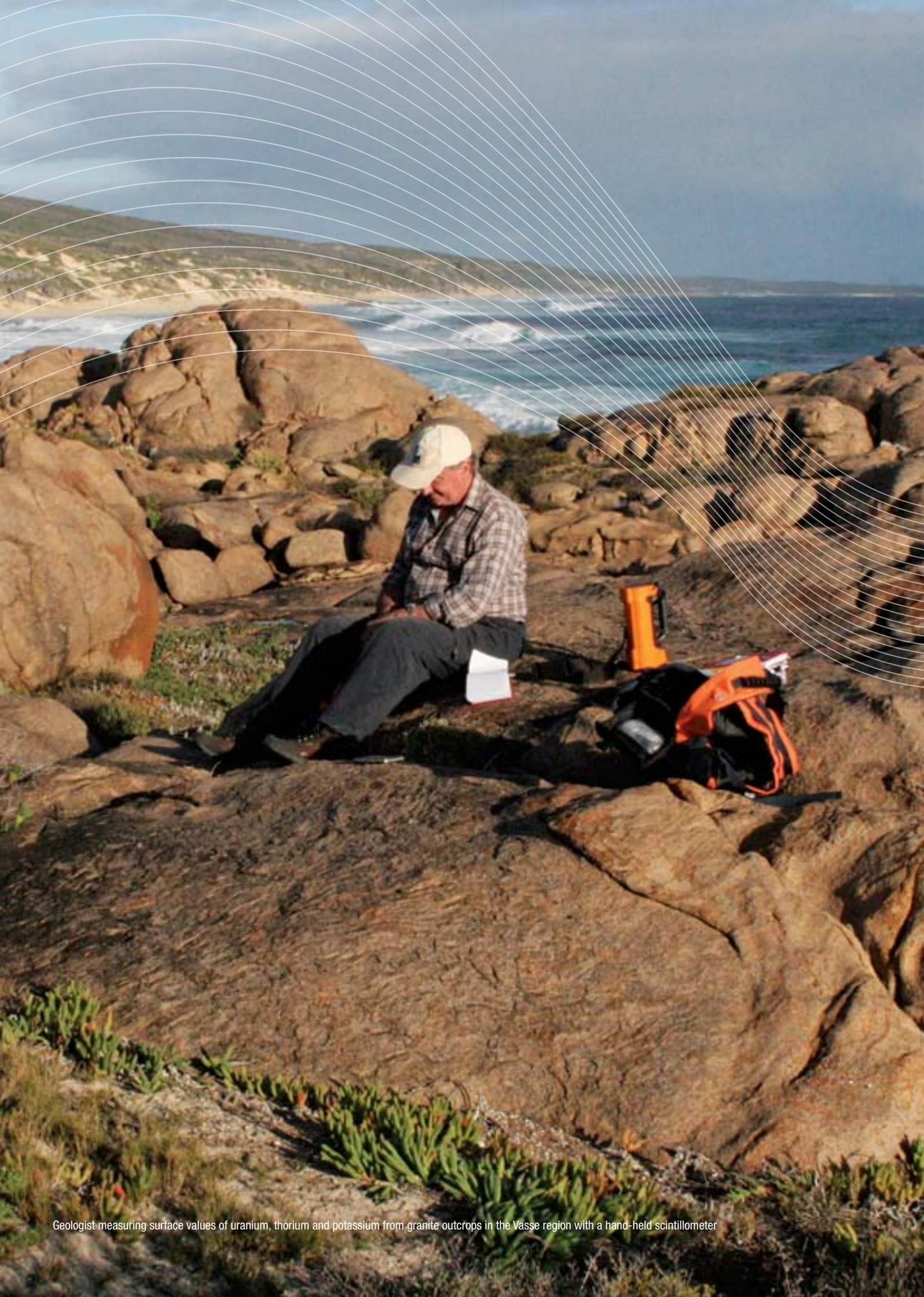
Geologist measuring surface values of uranium, thorium and potassium from granite outcrops in the Vasse region with a hand-held scintillometer
