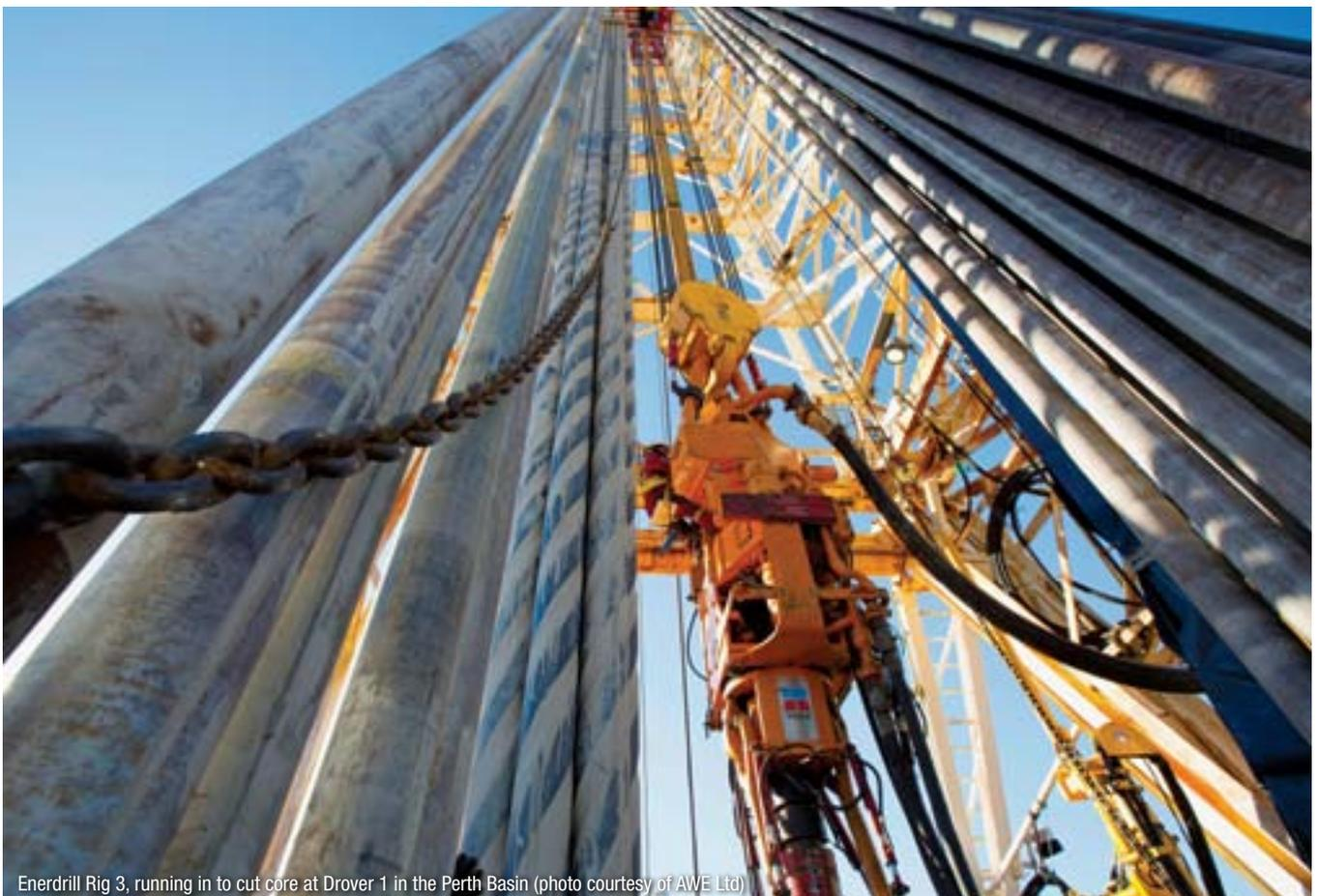
Enerdrill Rig 3, running in to cut core at Drover 1 in the Perth Basin (photo courtesy of AWE Ltd)
