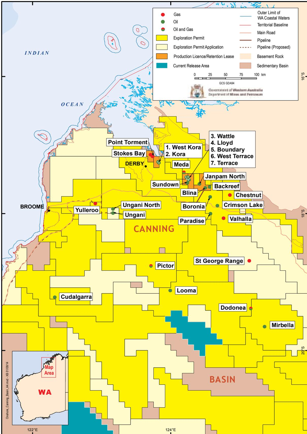
Figure 7. Significant hydrocarbon discoveries in the Canning Basin
