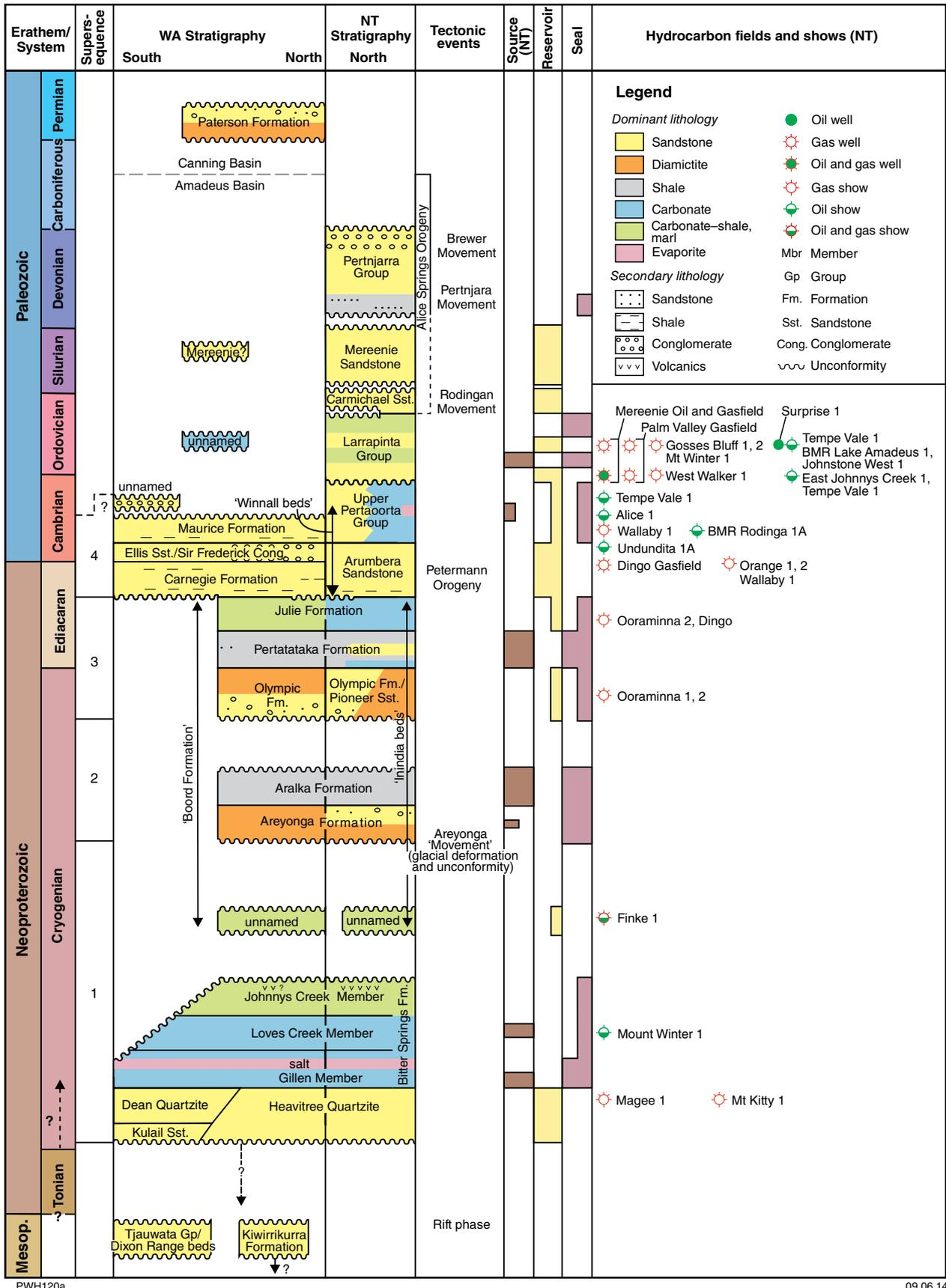
Figure 10. Stratigraphy, tectonic events, and hydrocarbon systems of the Amadeus Basin. Western Australian stratigraphy is compared with the northern Amadeus Basin stratigraphy of the Northern Territory. Source rock intervals are based on Northern Territory data. Exploration drilling is restricted to the Northern Territory
