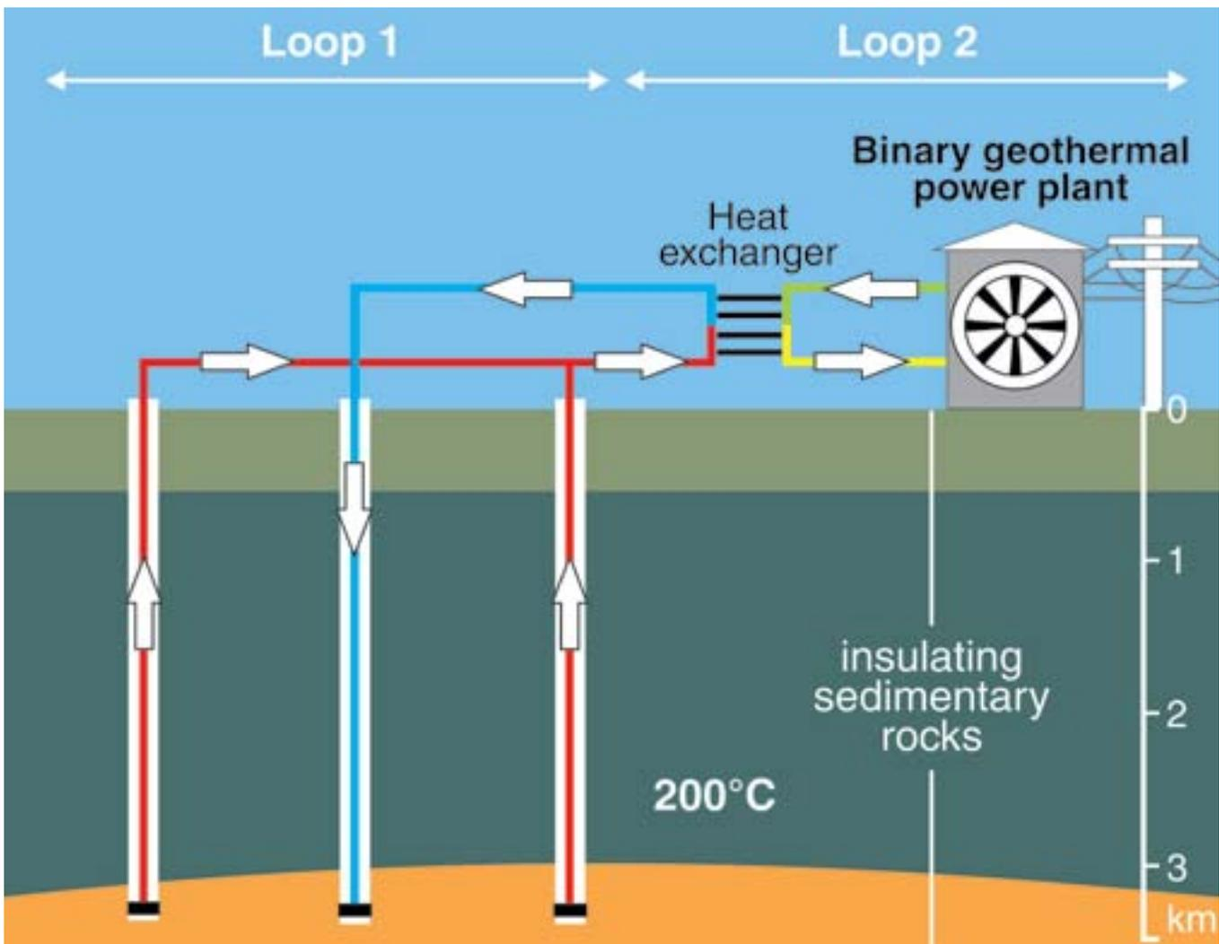
Figure 33. Example of binary cycle power plant, where the hot geothermal fluid is run through a “heat exchanger” and returned directly to the source reservoir. The turbine is run by a closed circuit “working fluid”
