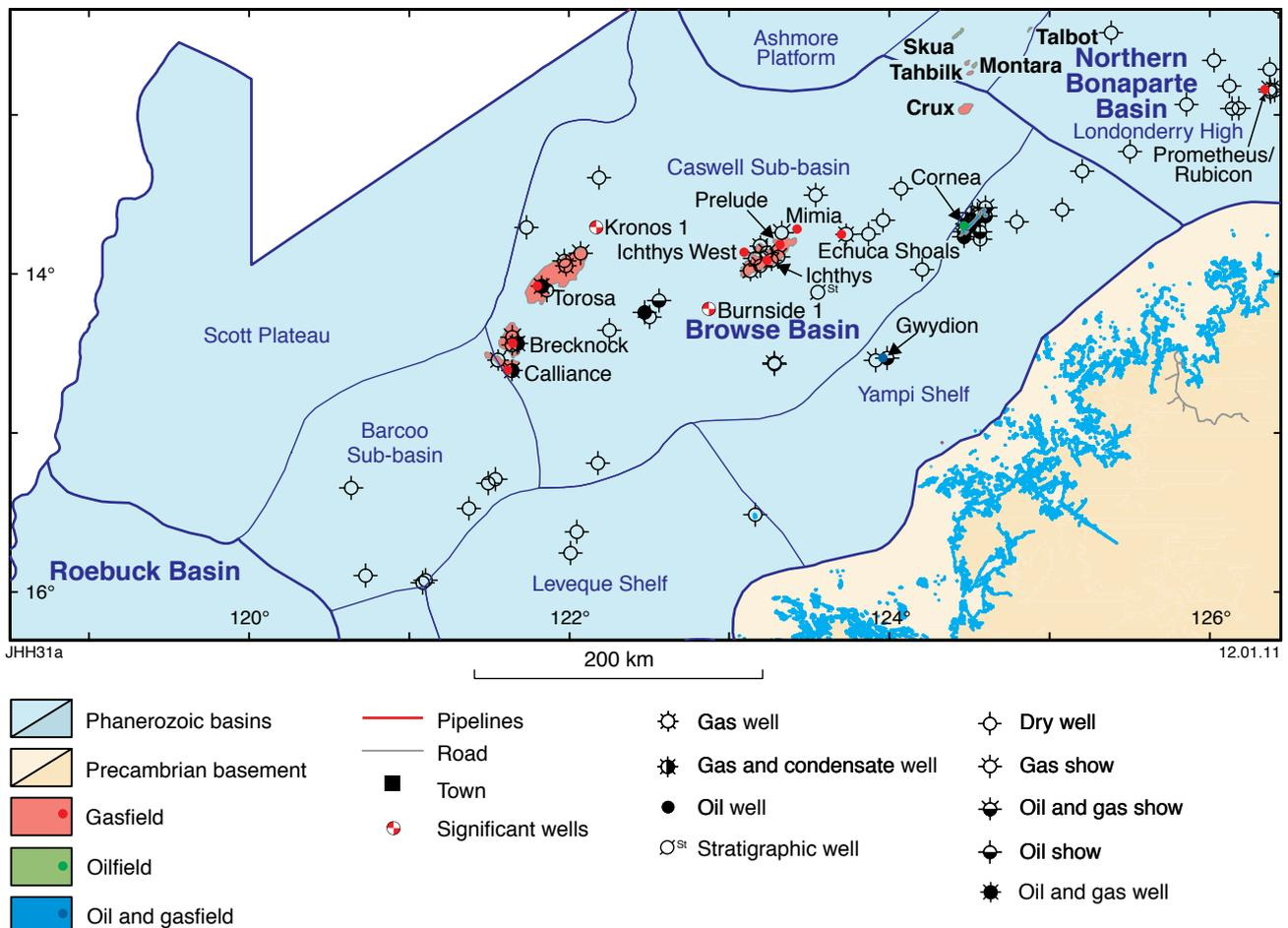
Figure 13. The Browse Basin, showing tectonic units, exploration wells and petroleum fields
