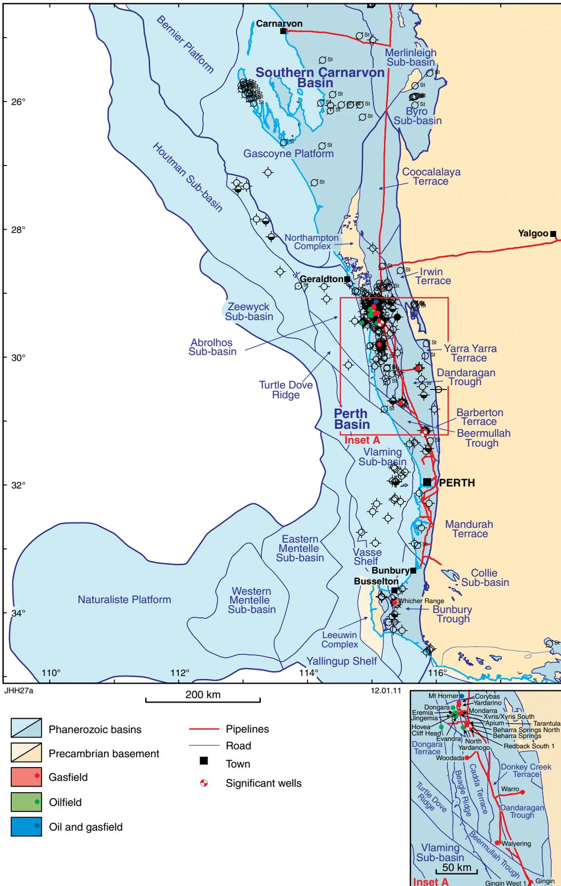
Figure 25. The Perth Basin, showing tectonic units, pipelines, fields, and petroleum wells
