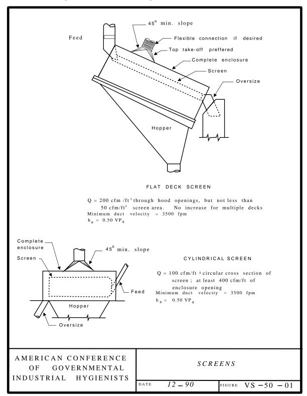
Figure A.6.: Schematic arrangement of dust collection chutes
