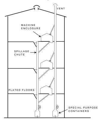
Figure 2.4.: Schematic arrangement of dust collection chutes.
