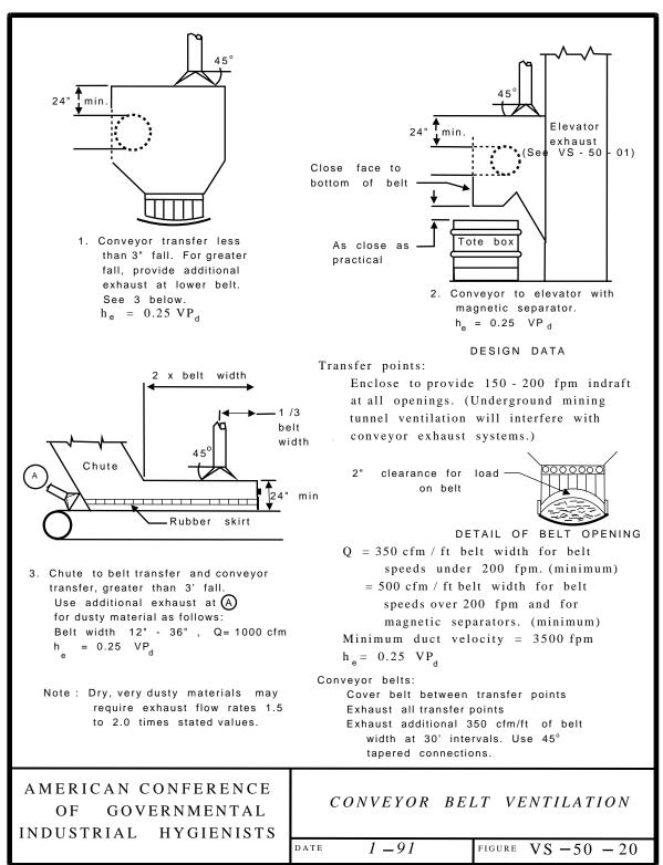
Figure A.5.: Schematic arrangement for ventilation with conveyor belts.
