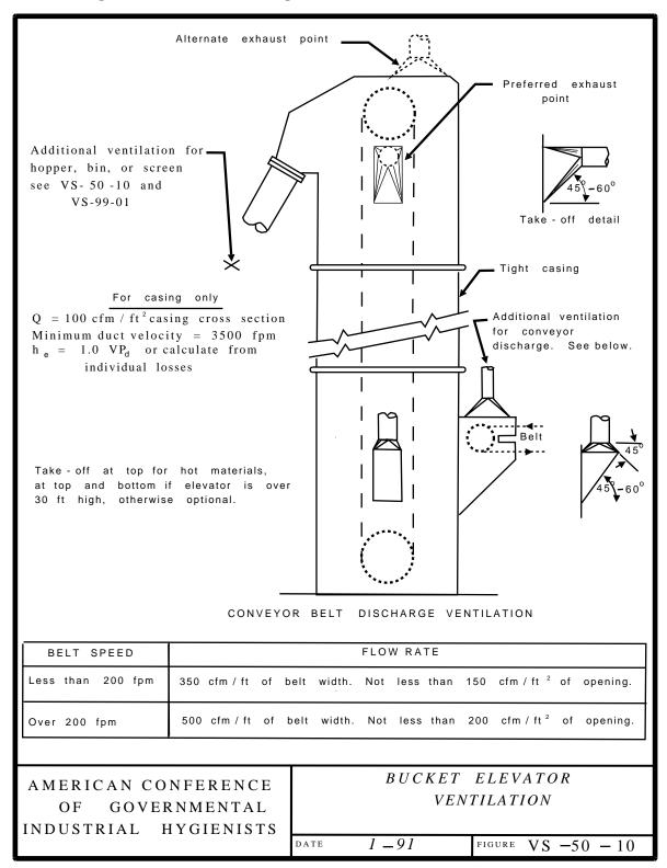
Figure A.4.: Schematic arrangement for ventilation in a bucket elevator.
