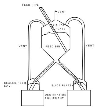
Figure 2.5.: Schematic arrangement for venting feed boxes into main bins.
