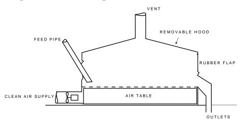
Figure 2.1.: Schematic arrangement for a vented hood over air table.
