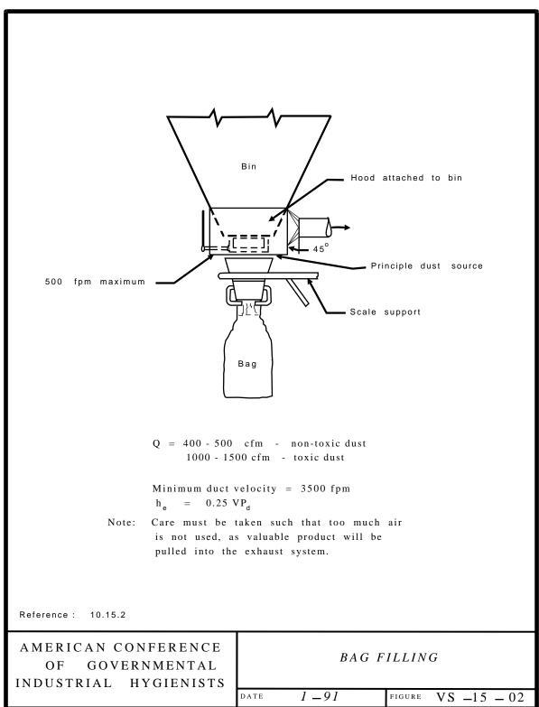
Figure A.1.: Schematic arrangement for ventilation in bag filling.
