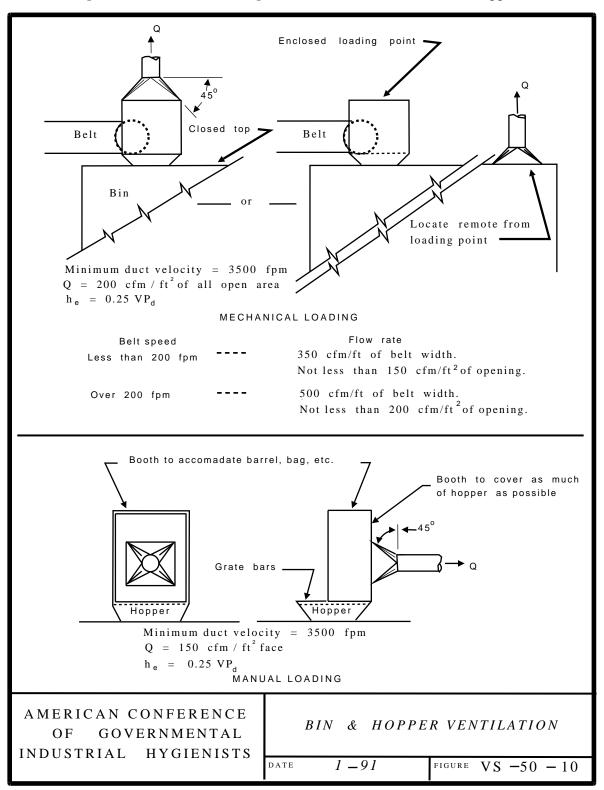
Figure A.3.: Schematic arrangement for ventilation in bins and hoppers.
