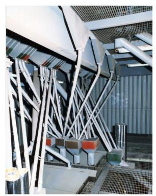
Figure B.7.: Feed distribution arrangement to HTRs – note enclosed feed hoppers, spillage collection hoppers and inspection doors
