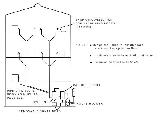
Figure 2.3.: Schematic arrangement of centralised vacuuming system.
