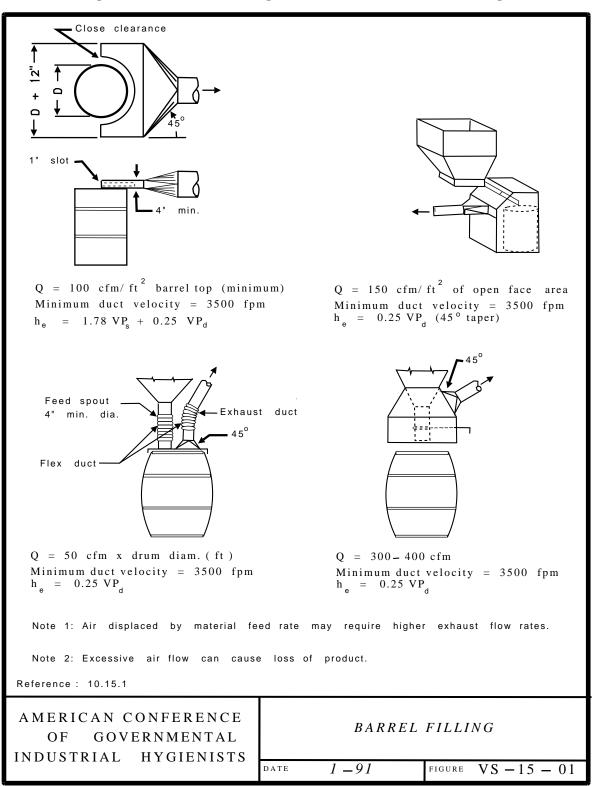
Figure A.2.: Schematic arrangement for ventilation in barrel filling.
