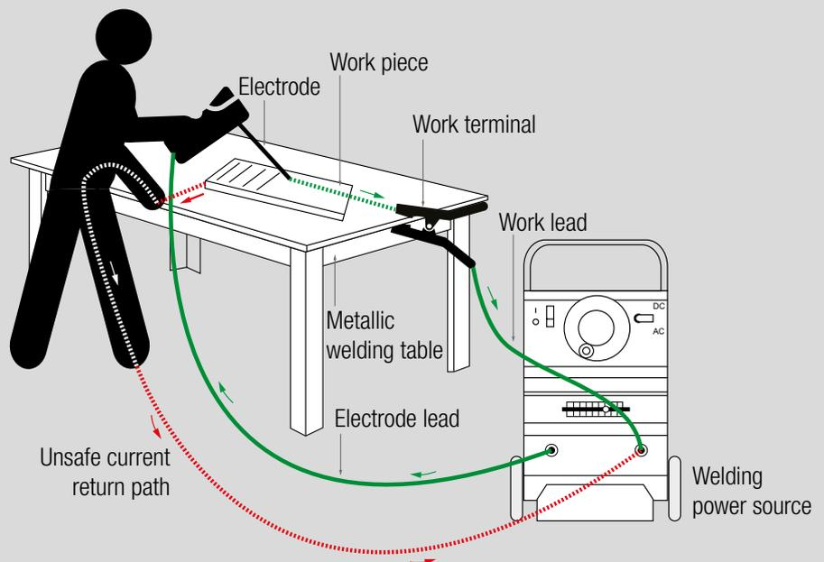
Example showing the safe current path (green) and unsafe current return path (red dots) if welder with inadequate PPE becomes part of the welding electrical circuit by touching the table
