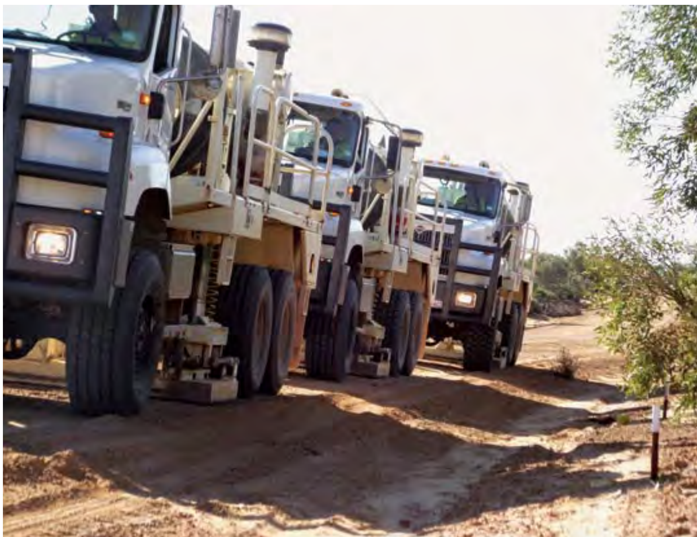
Vibroseis trucks passing cableless geophones on the Launer 2D seismic survey (Photo courtesy of Empire Oil and Gas)
