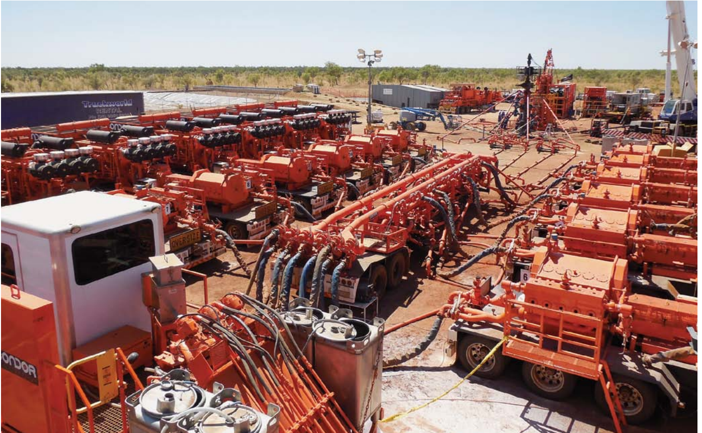
Hydraulic fracture stimulation equipment at Valhalla North 1 in the Canning Basin
