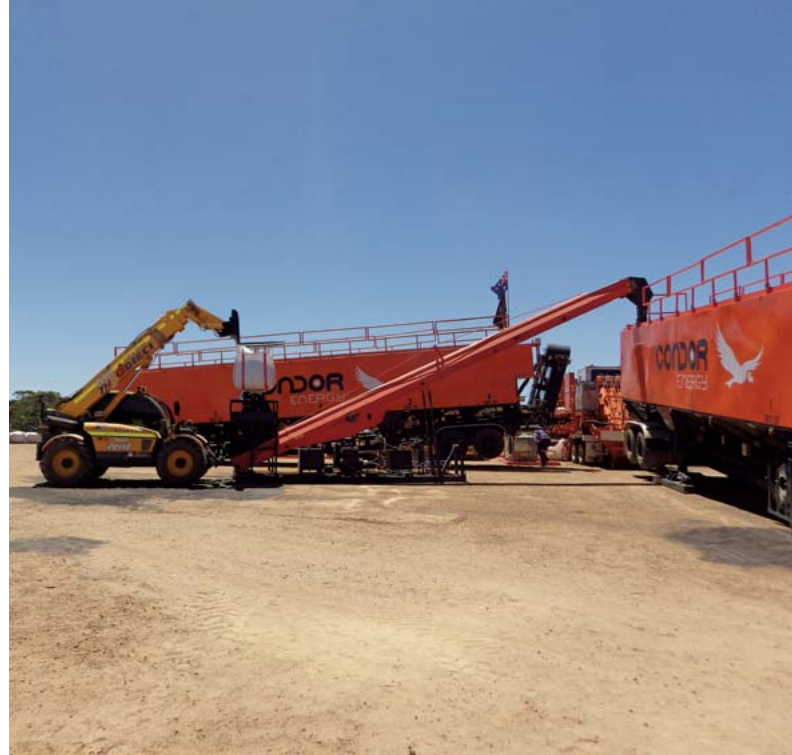
Loading proppant (sand) into the sand dragon prior to the fracture stimulation at Warro 5
