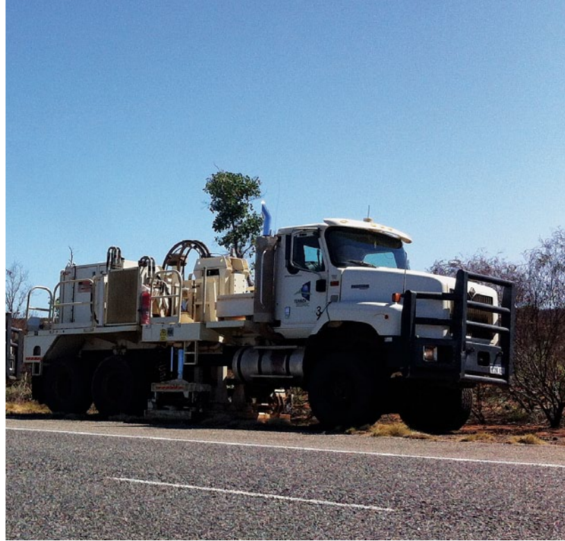
Vibroseis truck on the Canning Coastal seismic survey
