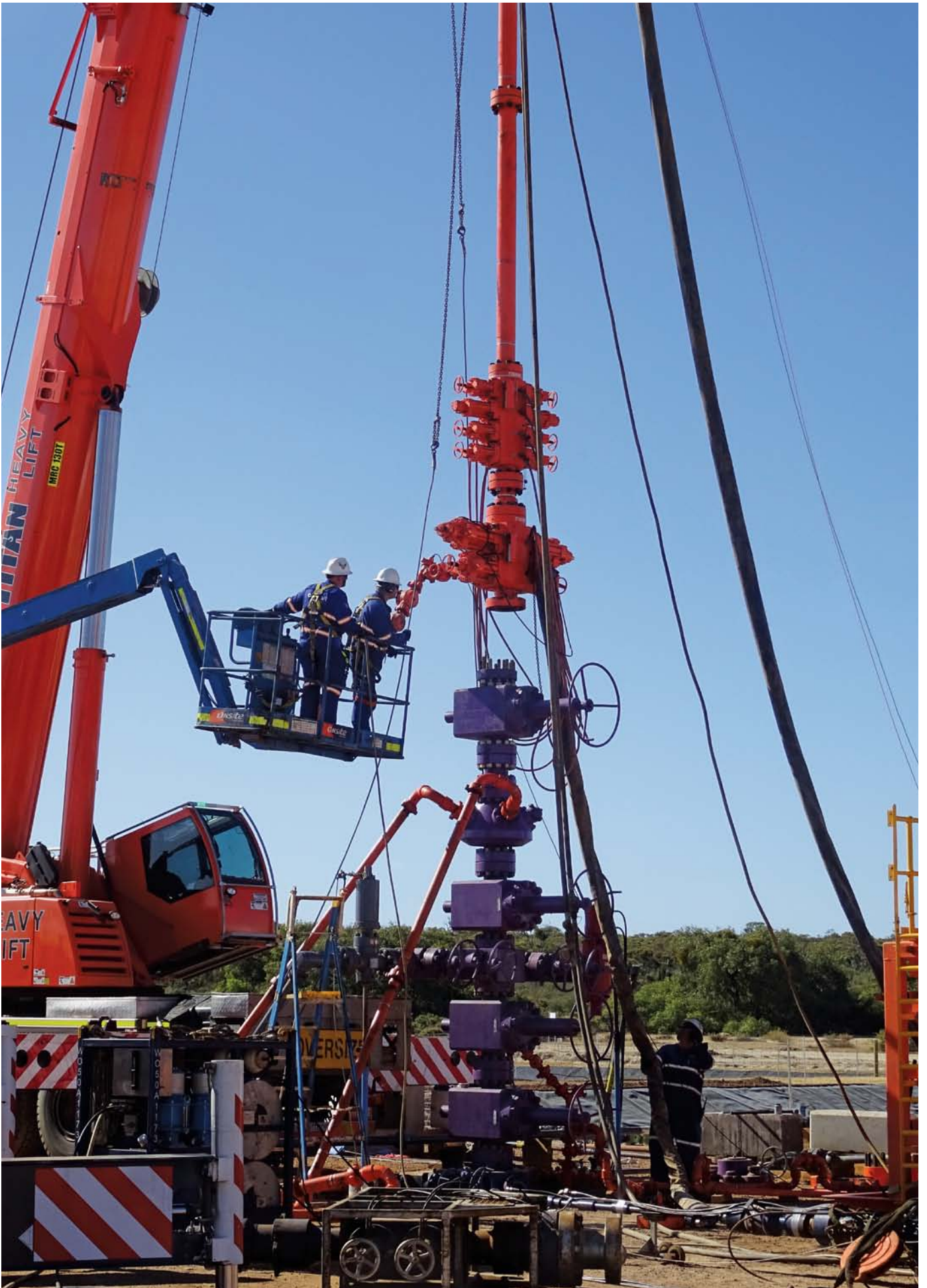
Rigging up coiled tubing on a frac tree at Warro 5
