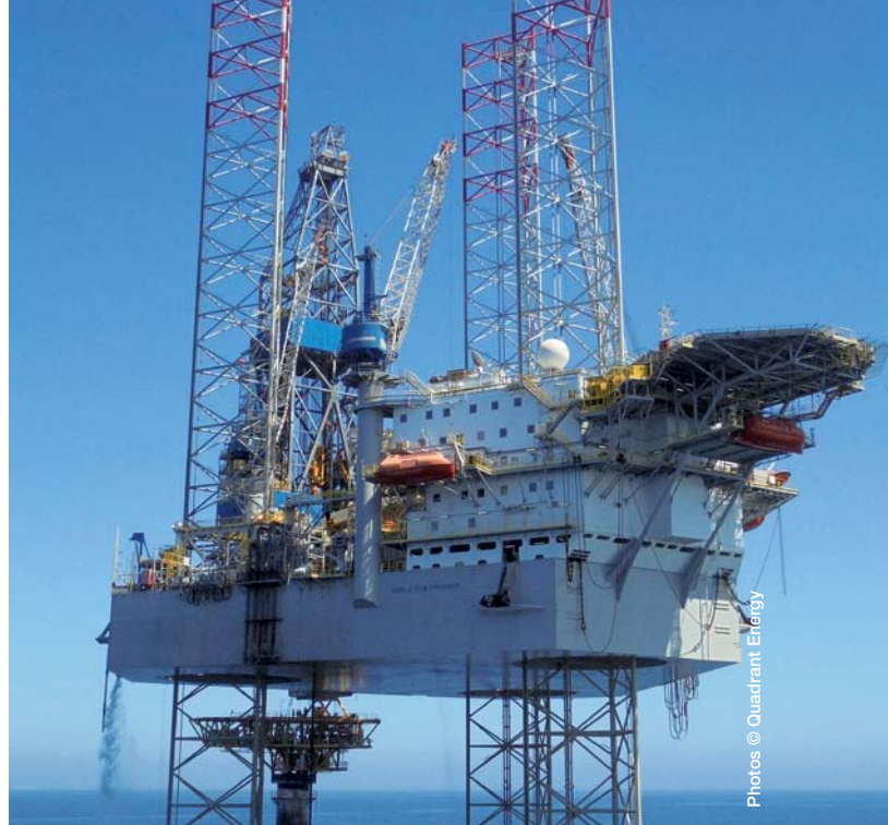
The Noble Tom Prosser jackup rig being utilised for decommissioning at the Harriet Charlie platform by Quadrant Energy
