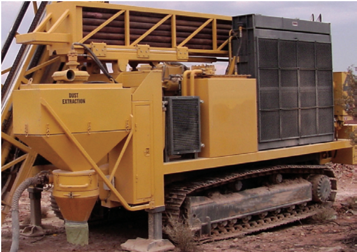
Figure 14.1 Example of a dust extraction system on an RC drill rig
