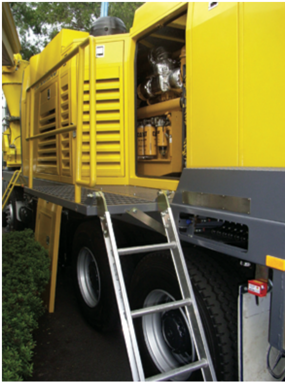
Figure 6.1 Example of enclosed engine and hydraulic system that minimises the potential for interaction with hot surfaces, and facilitates fire and noise suppression
