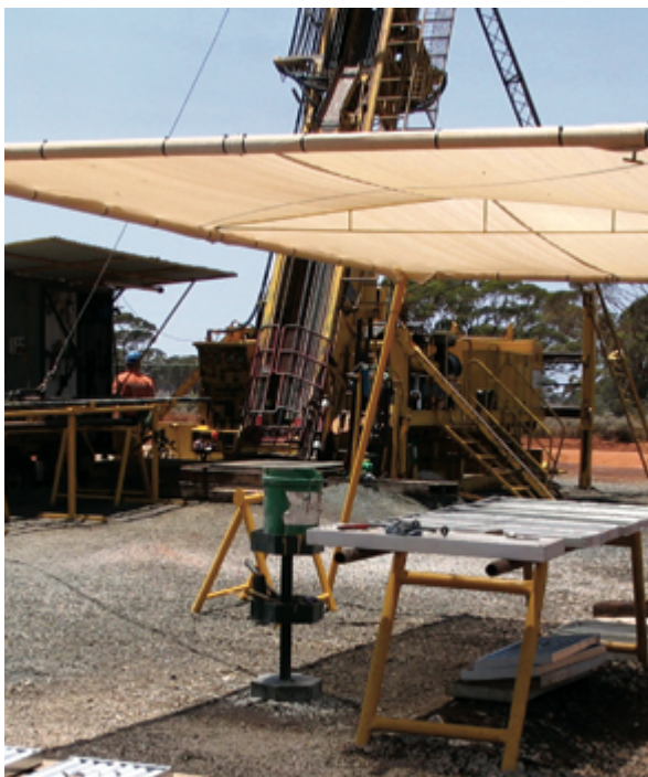
Figure 12.2 Example of shade shelter at a diamond core drill site
