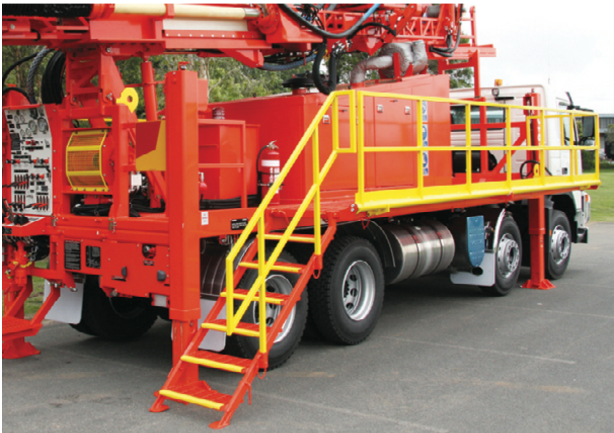
Figure 10.3 Example of steps, walkway and handrails for safe access to a drill rig
