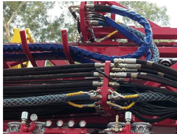
Figure 5.2 Example of full-length hose stockings and anchor points on an RC drill rig
