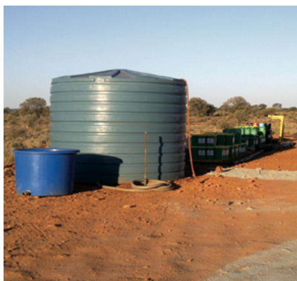
Figure 24.1 Example of well laid-out diamond core drill site showing designated storage area and use of crushed rock to minimise dust and improve underfoot conditions
