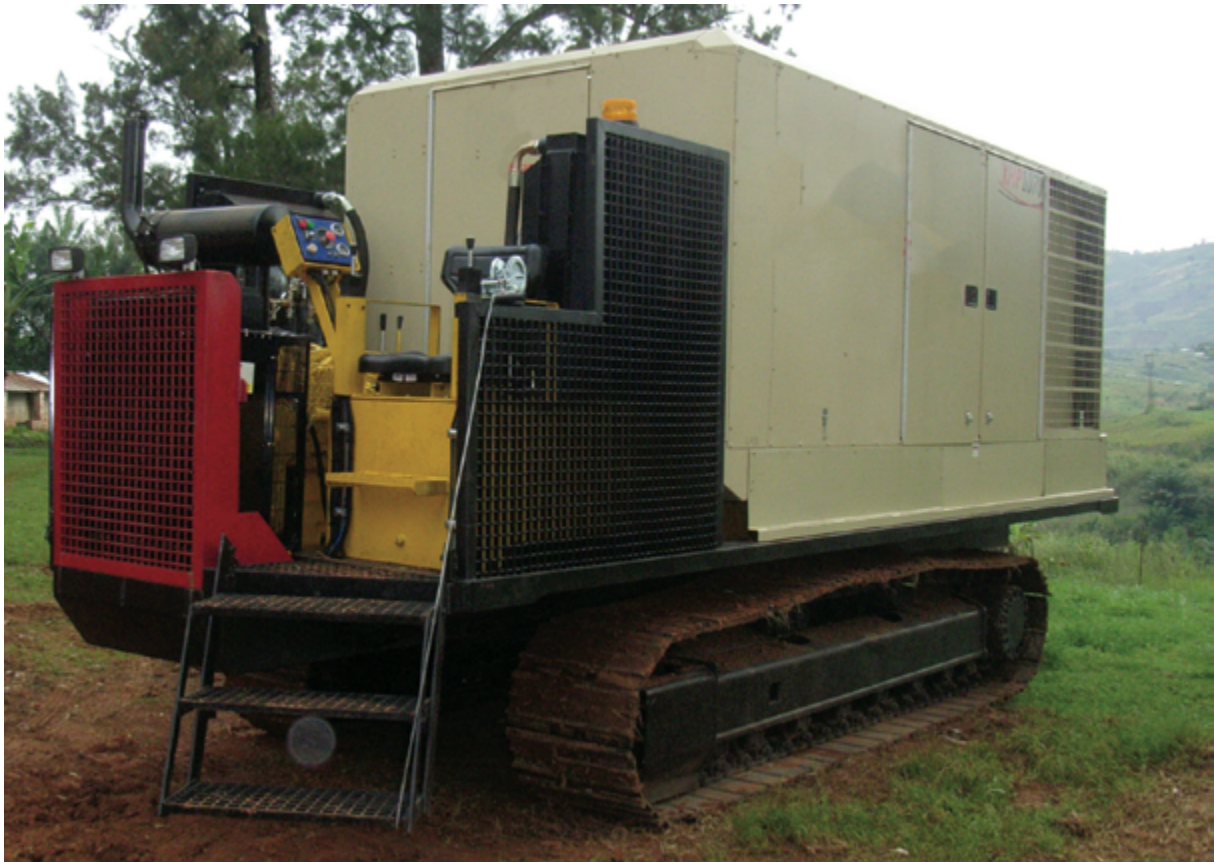
Figure 15.2 Example of noise suppression system on an air compressor
