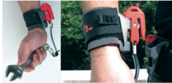
Figure 11.1 Example of tool lanyard that attaches to user's wrists or belt, and allows tools to be switched between hands while working at height
