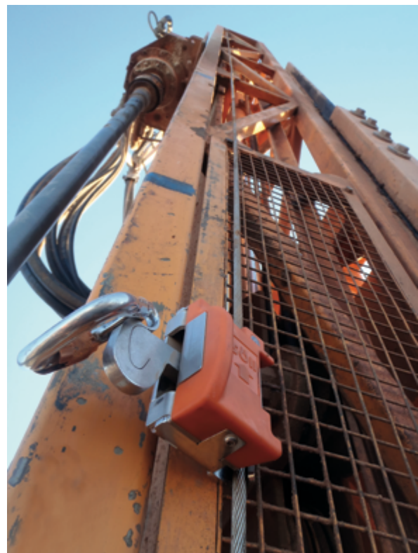
Figure 10.1 Example of static line and sliding brake fitted to mast of a drill rig
