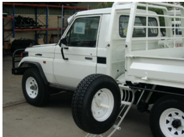
Figure 9.3 Example of tyre handler on a light vehicle
