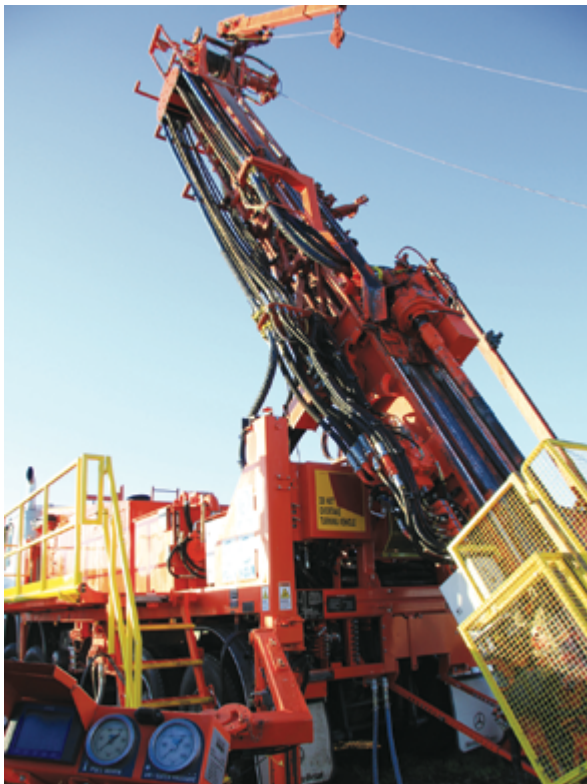
Figure 4.2 Example of remote control console in combination with guarding. The operator is removed from rotating and moving parts of the drill rig
