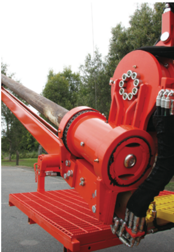
Figure 9.2 Closer view of rod handling arm shown in Figure 8.1
