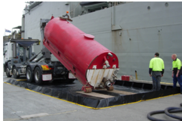
Figure 7.3 Example of drive-on bund
