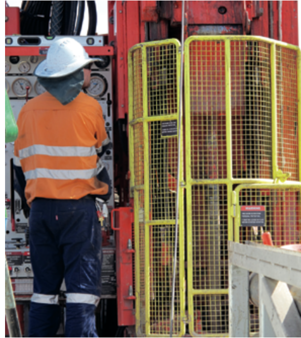
Figure 4.3 Example of effective guarding on a multipurpose drill rig
