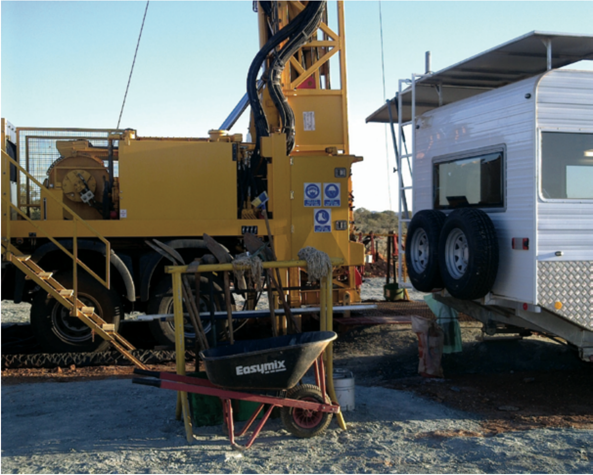
Figure 24.2 Example of well laid-out drill site showing tool racks and equipment storage
