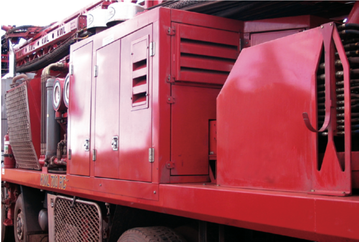
Figure 15.1 Example of an enclosure to suppress noise on a drill rig
