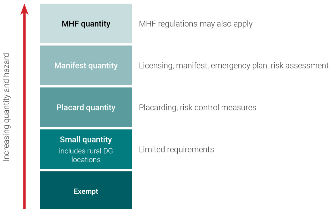
Figure 1 Schematic showing storage and handling regulatory regime
