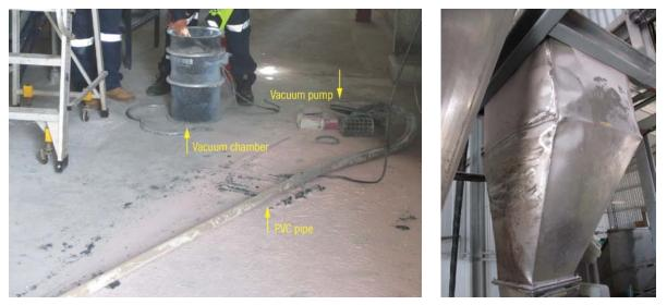
Damage to transfer system. Left. Vacuum pump chamber and pump, PVC transfer piping and evidence of spot fires on the floor. Right. Distortion of hopper caused by explosion.
