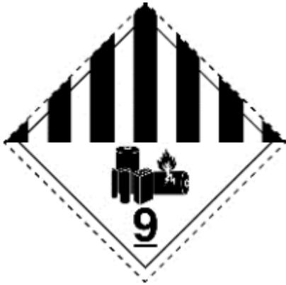
Figure 3 Class 9 label, model 9A for lithium batteries
