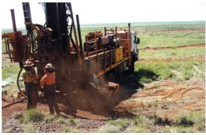
RC wet drilling (water injection)
