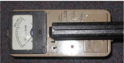
Figure B.1.: The Ludlum 12S meter reads in  $\mu R/h$
