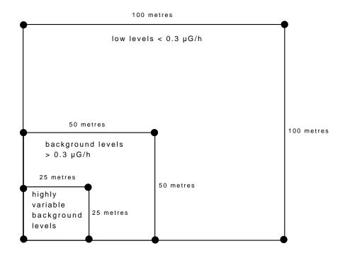
Figure 2.1.: Gamma survey – recommended grid sizes
