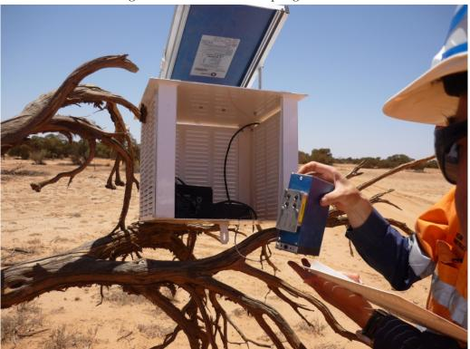
Figure 2.3.: Electronic sampling of radon
