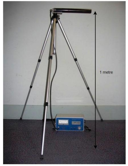
Figure 2.2.: Mini-Instruments 6-80 environmental radiation survey meter
