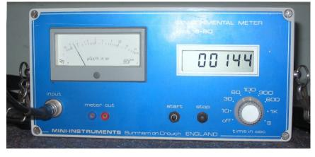
Figure B.2.: The Mini-Instruments environmental radiation survey meter reads in  $\mu$ Gy/h
