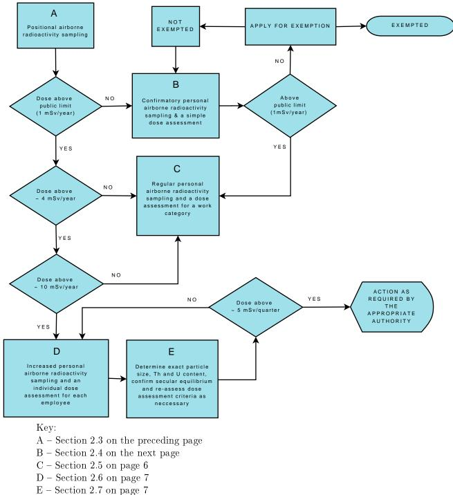
Figure 2.1.: Airborne radioactivity sampling
