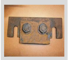
Photographs showing rail clamp as designed by original equipment manufacturer (top) and modified rail clamp (bottom) with open-ended slots and welded nuts and bolts
