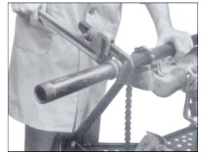
When using a RapidGrip wrench, be sure to center the work piece in the "v" of the hook. If the work piece is not in contact with both sides of the "v", it can reduce wrench gripping action and may result in failure of the hook.
