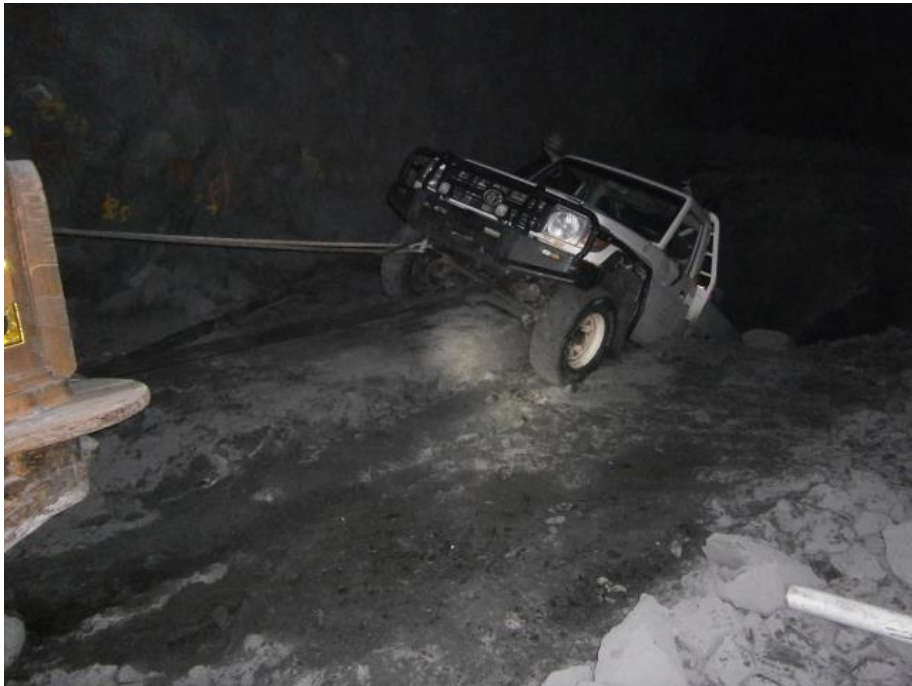
Light vehicle attached to loader with chain
