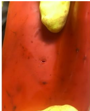
Left: Control transformer with exposed 1000V terminals. Centre: Tiny hole in glove. Right: Wrist of injured worker.
