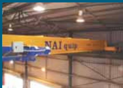
New 10 tonne NAI quip single beam crane
