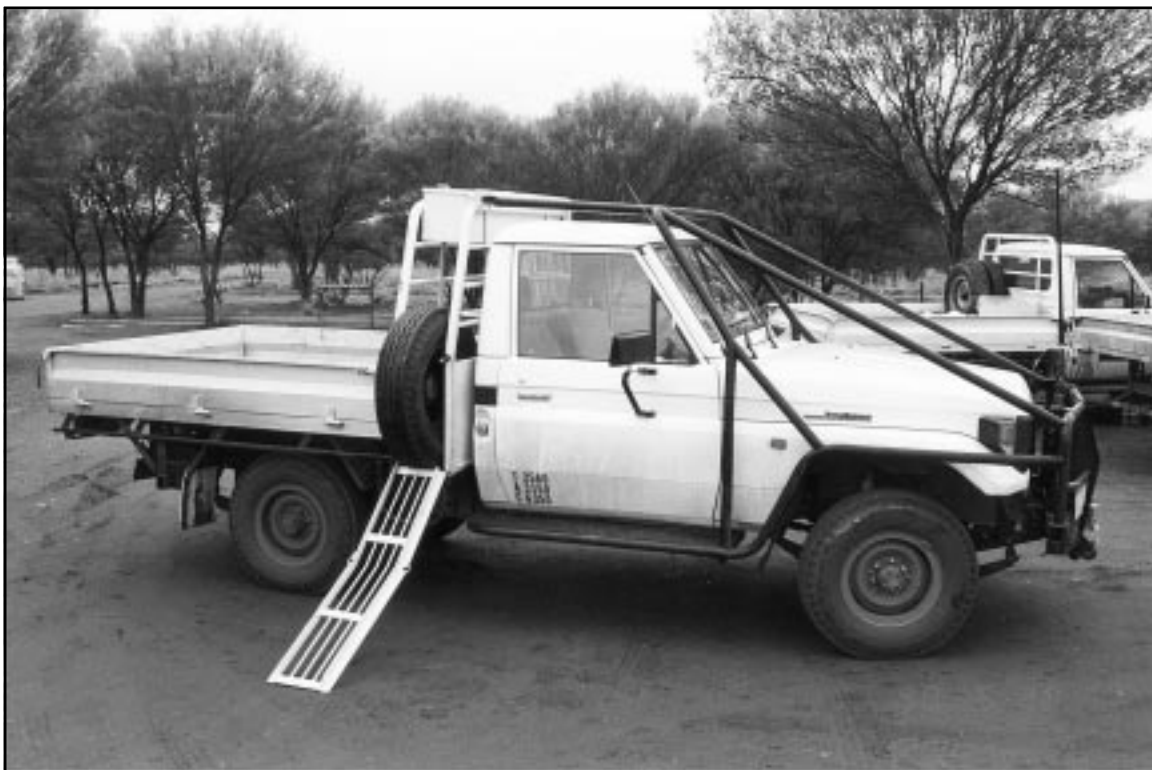
Tyre storage and side ramp to eliminate back strain / manual handling injury (Lawlers Gold Mine).
