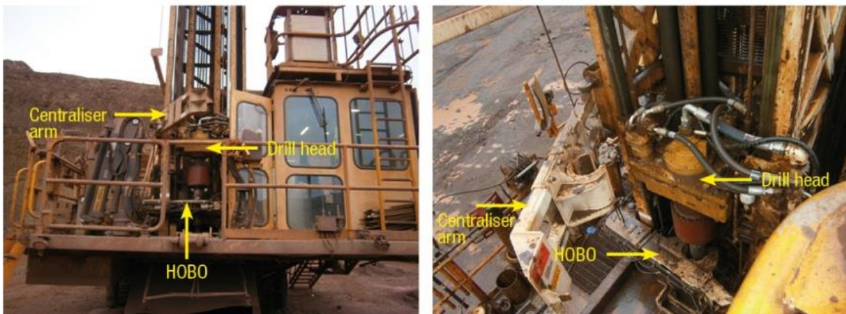
Blast-hole drill rig. Left. Front view showing position of HOB0, drill head, centraliser arm and drill cab. Right. Top view showing potential crush zone between the drill rod centraliser arm and drill head.
